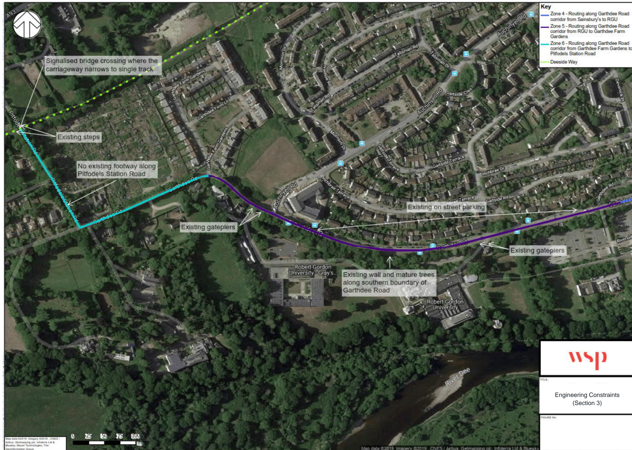
Figure 3-27 - Engineering Constraints (Section 3)
